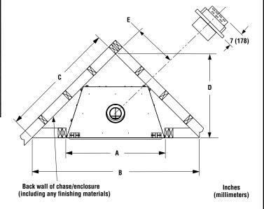
Figure 14 - Corner Framing with Horizontal Termination
